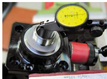
Output End Inspection
