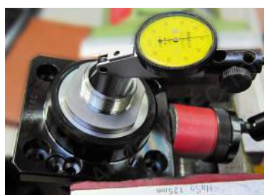
Output End Inspection
